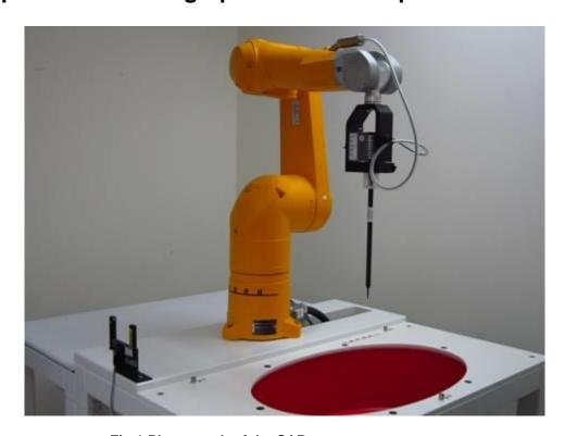
Fig.1 Photograph of the SAR measurement system
