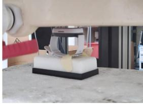
Fig.4 Front side of EUT to flat phantom
