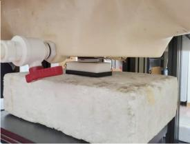
Fig.3 Back side of EUT to flat phantom
