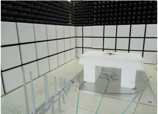
Radiated Emission Set up Photos (Above 1GHz)
