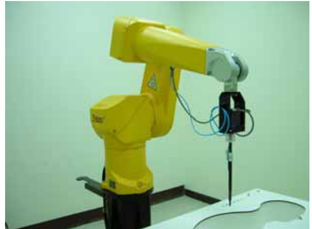
Fig. 5.2 Probe setup on robot
