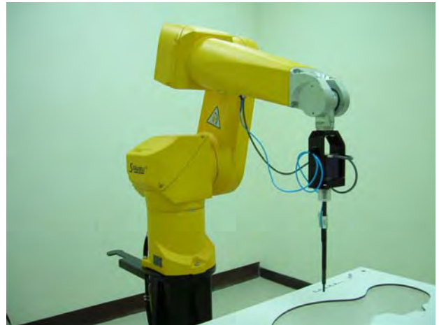
Fig. 5.2 Probe setup on robot
