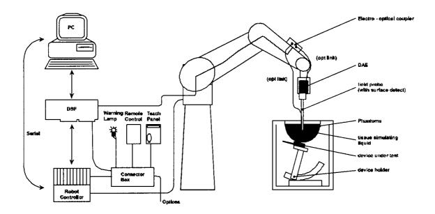
The DASY3 system for performing compliance tests consists of the following items:
