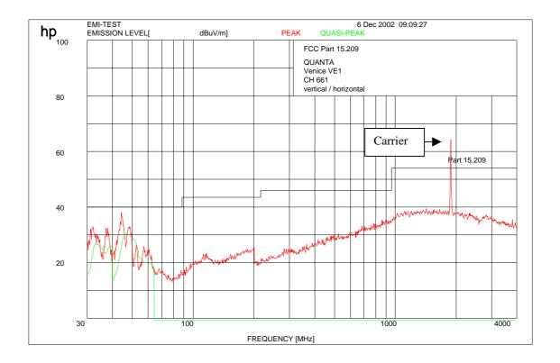
Carrier suppressed with a band rejection filter
