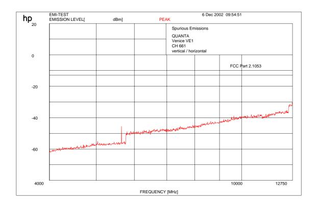
Carrier suppressed with a band rejection filter
