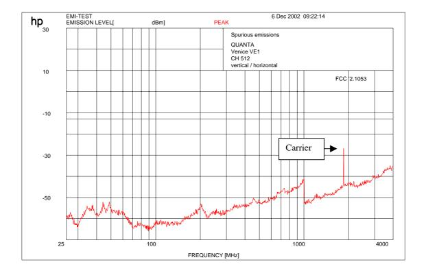
Carrier suppressed with a band rejection filter
