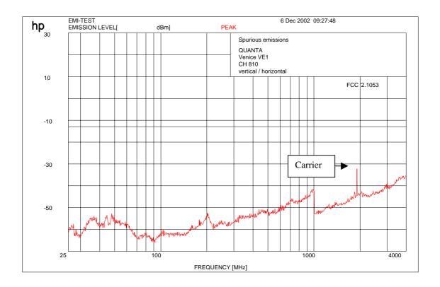
Carrier suppressed with a band rejection filter
