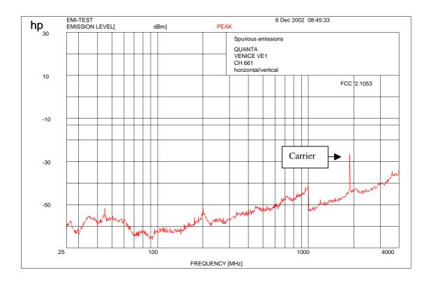
Carrier suppressed with a band rejection filter
