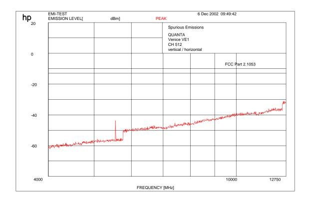
Carrier suppressed with a band rejection filter
