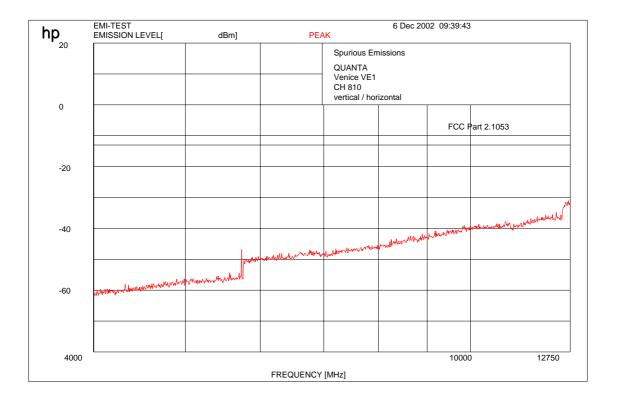
Carrier suppressed with a band rejection filter
