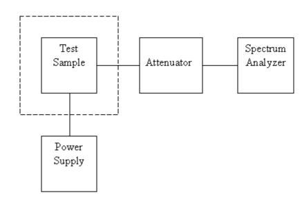
PS : Attenuator + Calbe Loss = 20.3 dB
