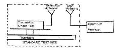
b) Raise and lower the test antenna from 1m to 4m and rotate turntable from 0° to 360°. Record the highest received signal showed in spectrum analyzer in dBuV as Rt . Calculate electric field strength in receive antenna in dBuV/m as Et. Et = Rt + AF
