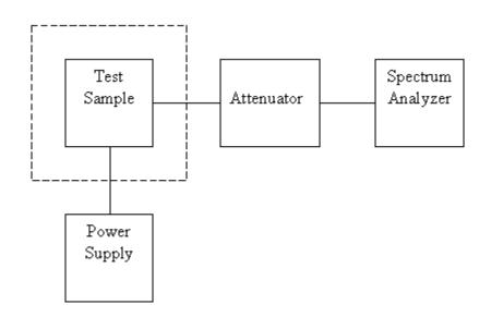
PS : Attenuator + Cable Loss = 20.3 dB
