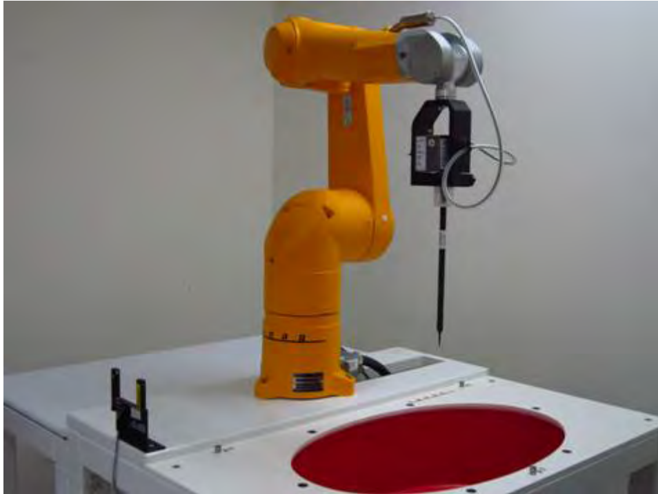
Fig.1 Photograph of the SAR measurement system
