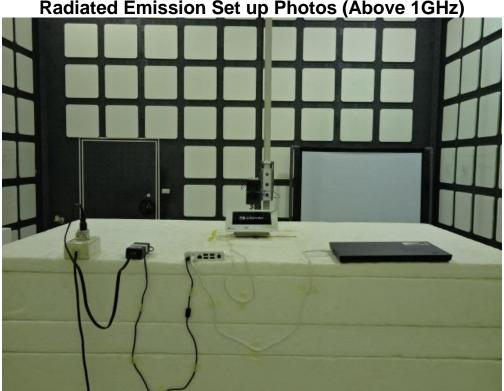
Radiated Emission Set up Photos (Above 1GHz)
