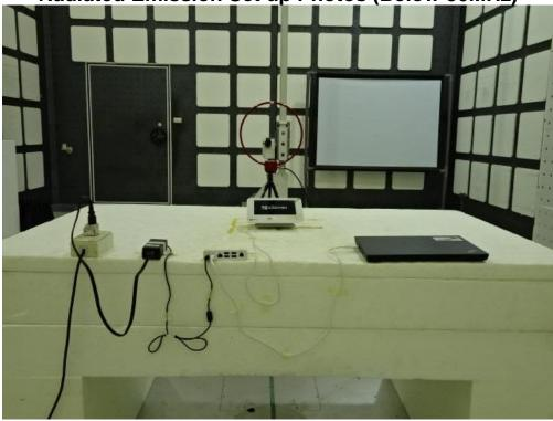
Radiated Emission Set up Photos (Below 1GHz)
