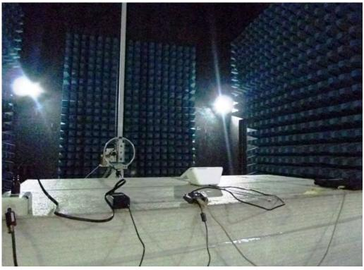
Radiated Emission Set up Photos (Below 1GHz)
