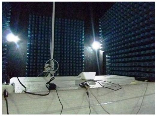
Radiated Emission Set up Photos (Below 1GHz)
