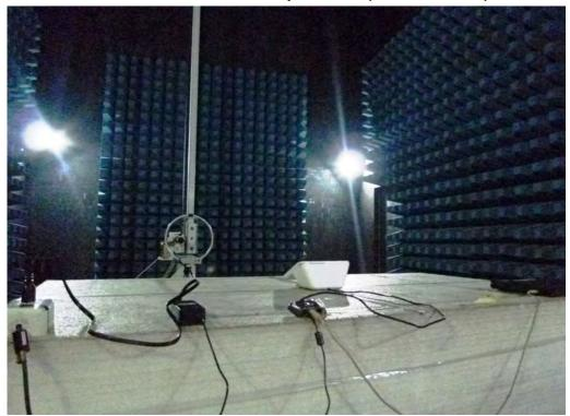
Radiated Emission Set up Photos (Below 1GHz)
