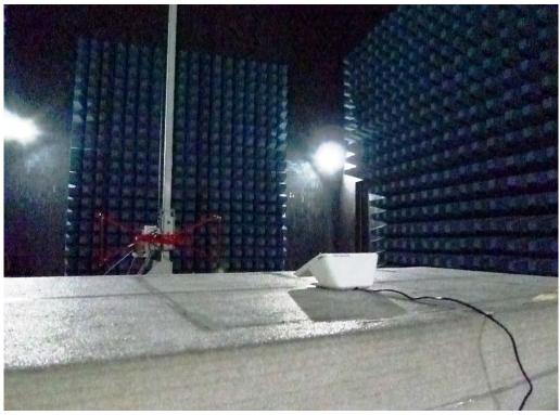
Radiated Emission Set up Photos (Above 1GHz)
