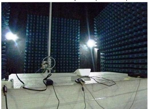
Radiated Emission Set up Photos (Below 1GHz)
