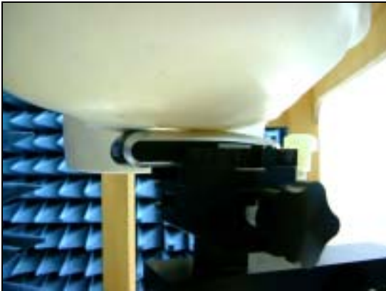
Figure 12. Left Head SAR Test Setup (Cheek)
