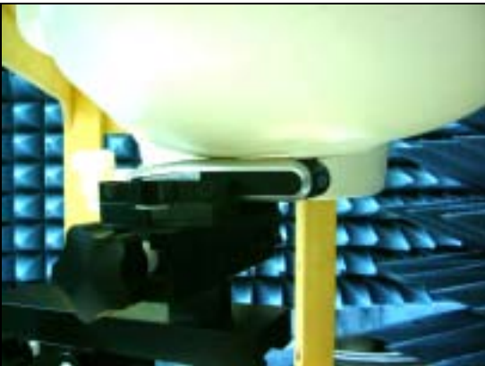
Figure 14. Right Head SAR Test Setup (Cheek)
