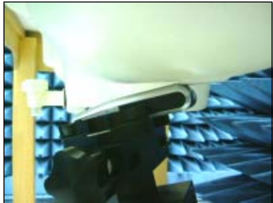
Figure 15. Right Head SAR Test Setup (Tilted)
