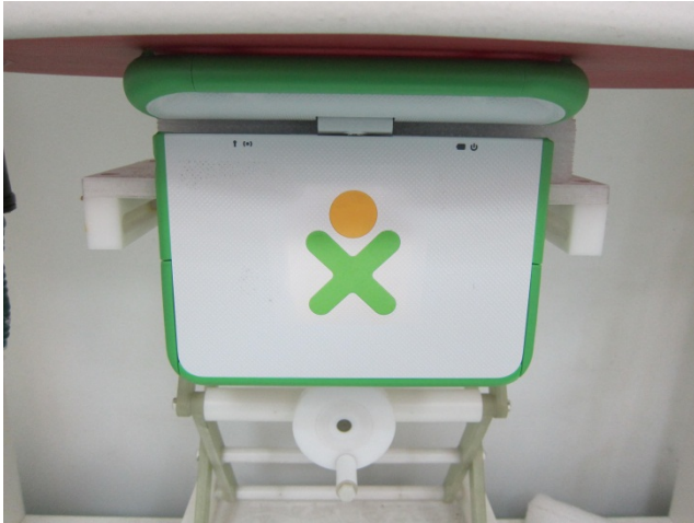
Bottom of Laptop with Phantom 0 cm Gap – Antenna Position 0°
