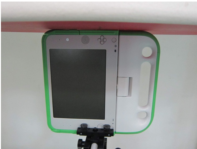
Edge2 with Phantom 0 cm – Antenna Position 0°
