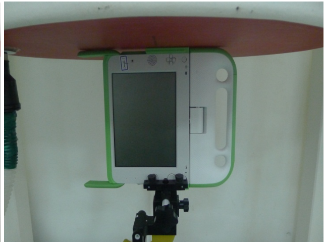
Edge2 with Phantom 0 cm – Antenna Position 180°
