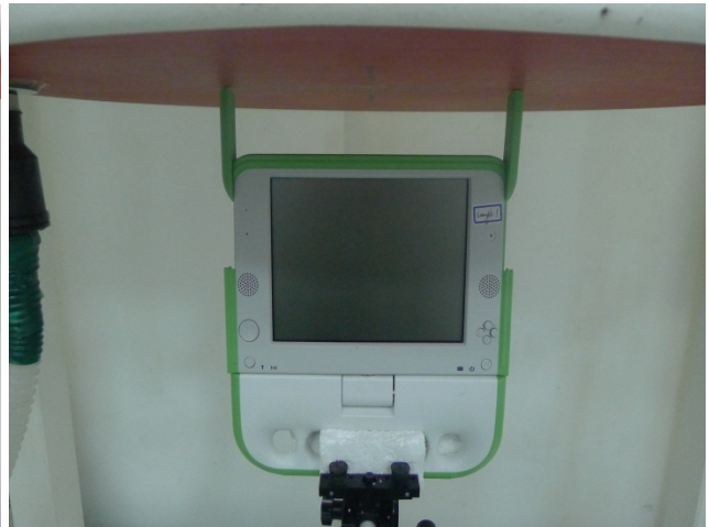
Edge1 with Phantom 0 cm – Antenna Position 180°
