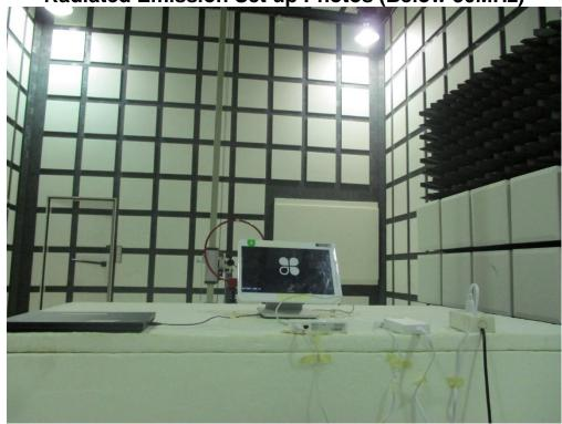
Radiated Emission Set up Photos (Below 1GHz)
