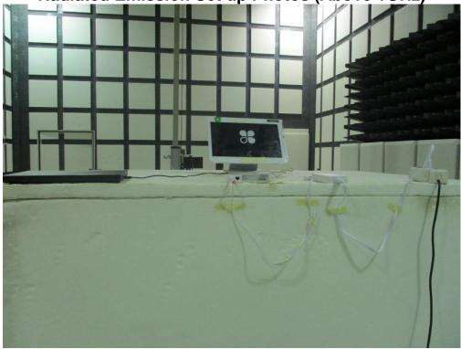
Radiated Emission Set up Photos (Front View)
