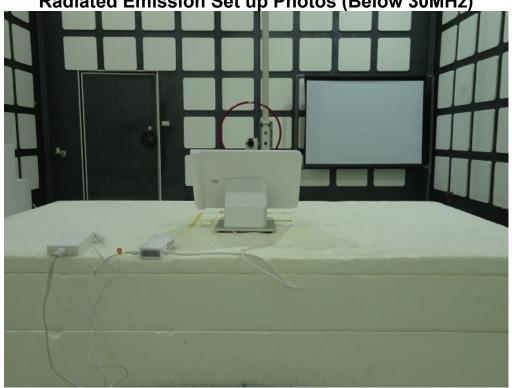
Radiated Emission Set up Photos (Below 1GHz)
