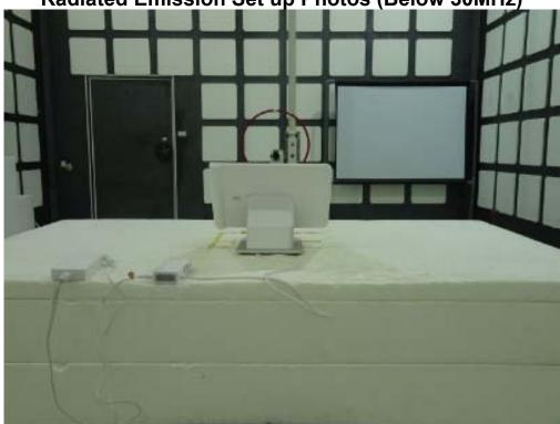
Radiated Emission Set up Photos (Below 1GHz)
