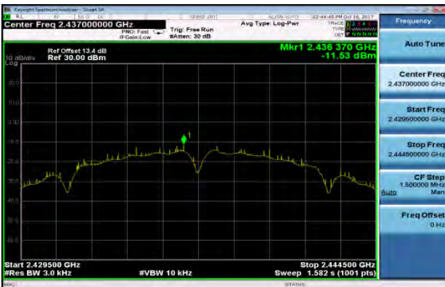
Power Spectral Density Test Plot (CH-High)
