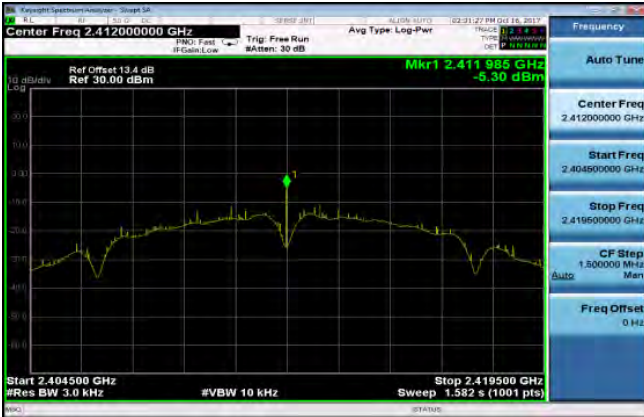
Power Spectral Density Test Plot (CH-Mid)
