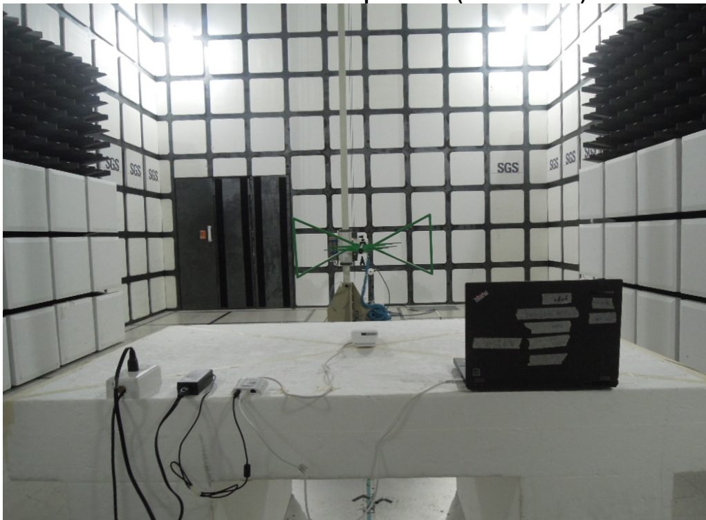
Radiated Emission Set up Photos (Below 1GHz)
