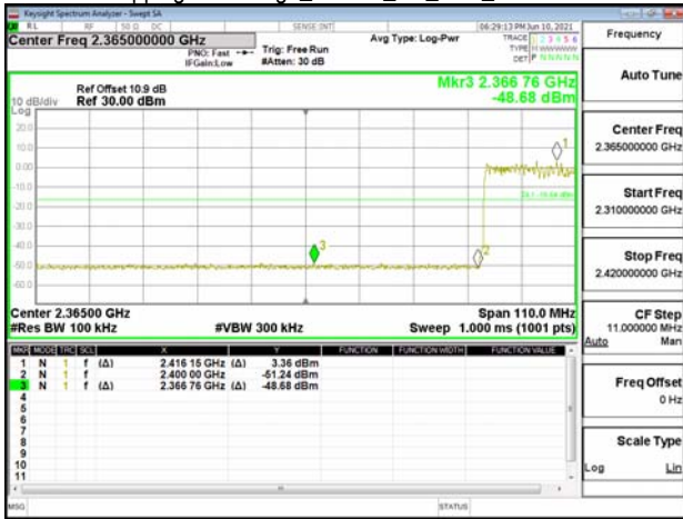
Hopping Band Edge_8DPSK_3M_DH5_2480MHz
