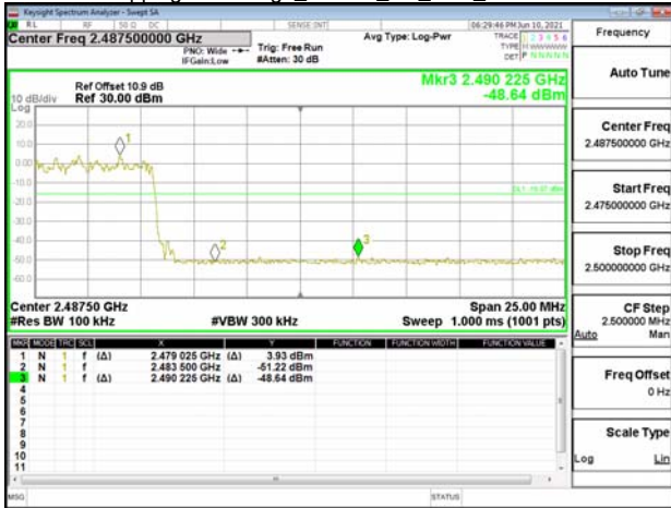
Hopping Band Edge_8DPSK_3M_DH5_2480MHz
