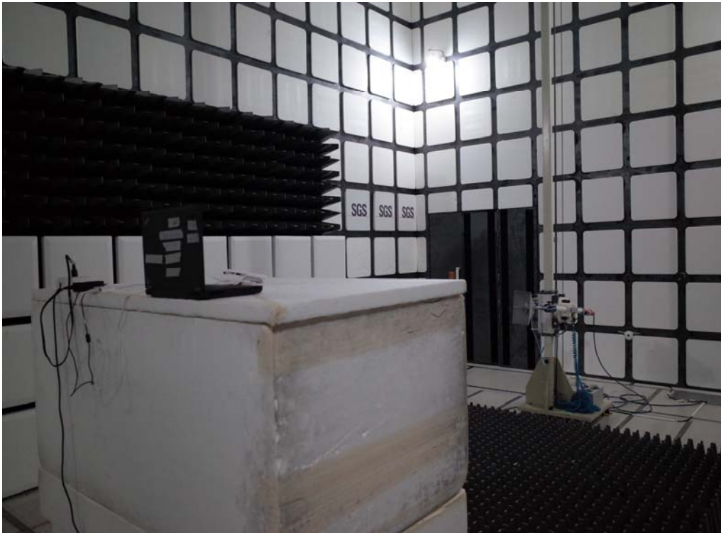
Radiated Emission Set up Photos (Front View)
