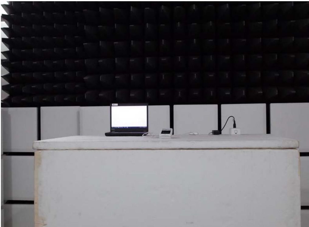
Radiated Emission Set up Photos (Front View)
