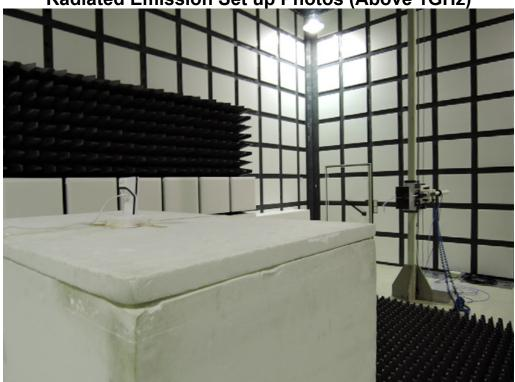
Radiated Emission Set up Photos (Front View)
