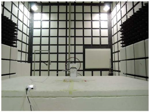
Radiated Emission Set up Photos (Below 1GHz)
