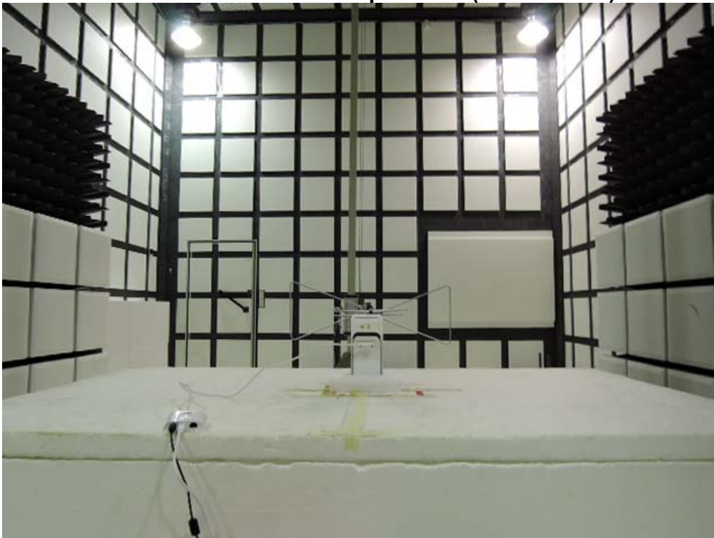
Radiated Emission Set up Photos (Below 1GHz)
