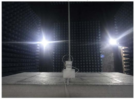
Radiated Emission Set up Photos (Below 1GHz)
