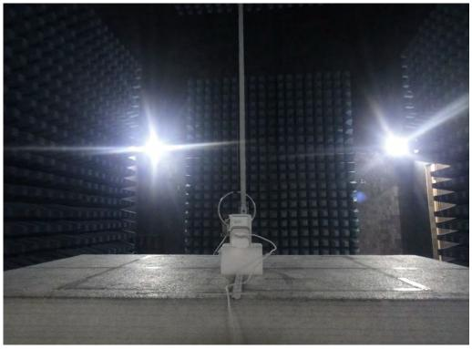
Radiated Emission Set up Photos (Below 1GHz)
