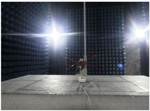
Radiated Emission Set up Photos (Above 1GHz)
