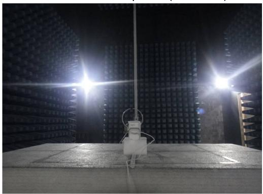
Radiated Emission Set up Photos (Below 1GHz)
