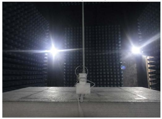
Radiated Emission Set up Photos (Below 1GHz)
