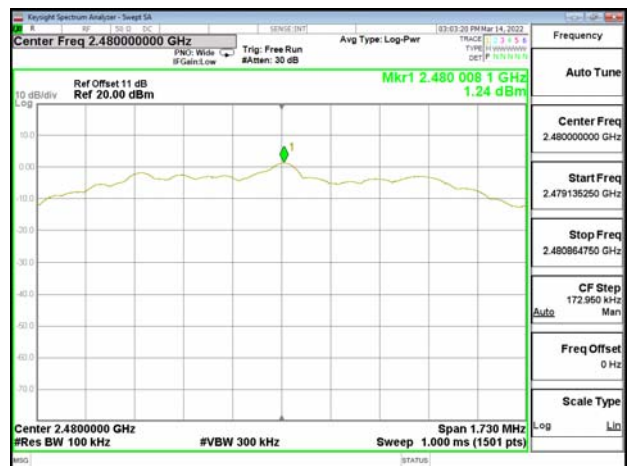
Reference Level_BLE 2M_HighCH39-2480MHz
