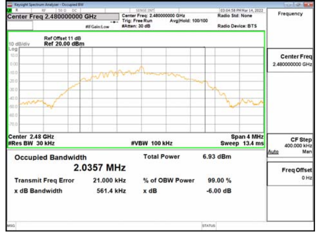
IC OBW_BLE 2M_HighCH39-2480MHz
