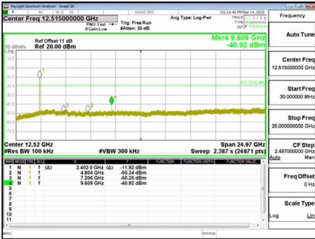
Spurious Emission_BLE 1M_MidCH20-2442MHz
