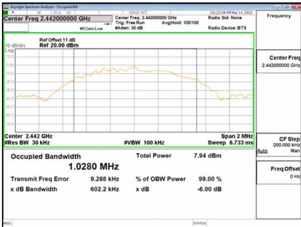
IC OBW_BLE 1M_HighCH39-2480MHz
