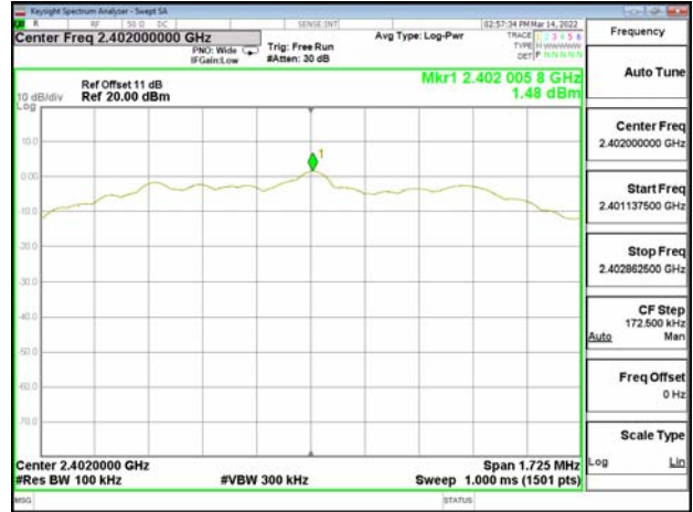
Reference Level_BLE 2M_MidCH20-2442MHz
