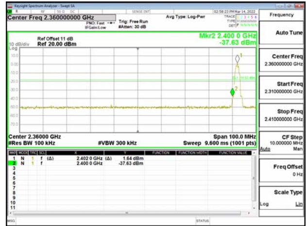
Band Edge_BLE 2M_HighCH39-2480MHz
