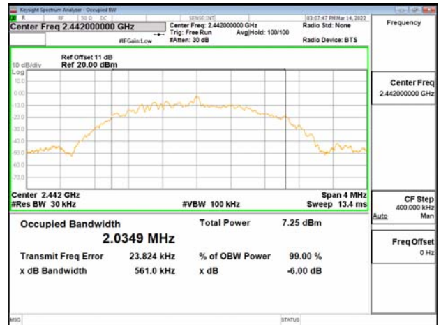
IC OBW_BLE 2M_HighCH39-2480MHz
