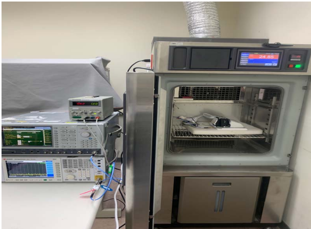
Conducted Setup Photo (Measurement at Antenna Port)
