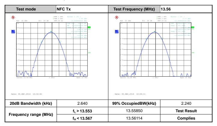
B.1 Test Result of 20dB Spectrum Bandwidth
