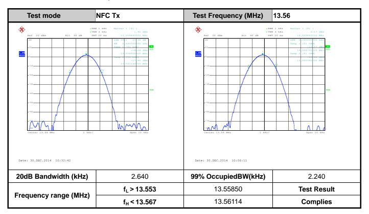
B.1 Test Result of 20dB Spectrum Bandwidth
