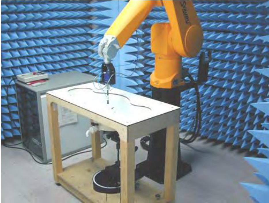
Fig.1 Photograph of the SAR measurement System
