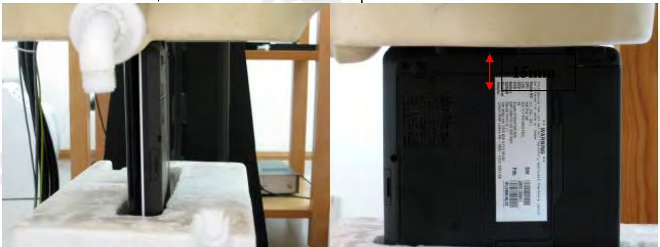
Fig.6 Left side of Notebook is paralleled with flat phantom, panel pointing out of Notebook, and and Notebook contact with flat phantom.
