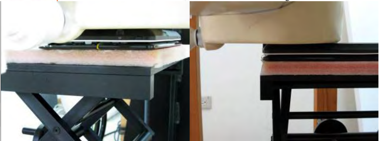
Fig.5 Bottom side of the Notebook is paralleled with panel and flat phantom, panel is pointing out of Notebook, bottom face is contact flat phantom.
