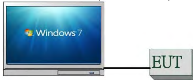
Fig. 2-2 Conducted Emission (AC Power Line) Configuration
