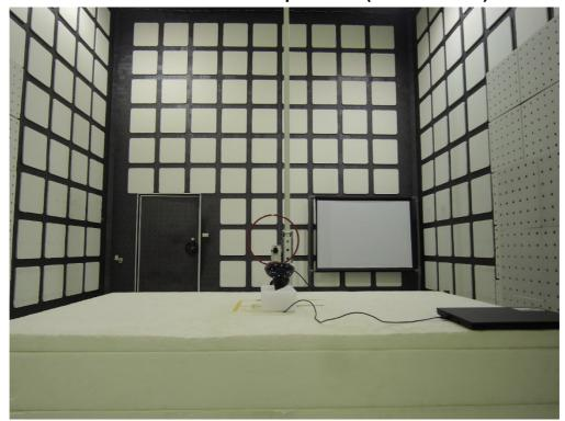
Radiated Emission Set up Photos (Below 1GHz)
