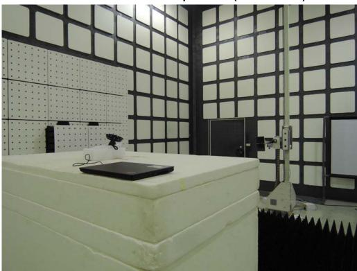
Radiated Emission Set up Photos (Front View)
