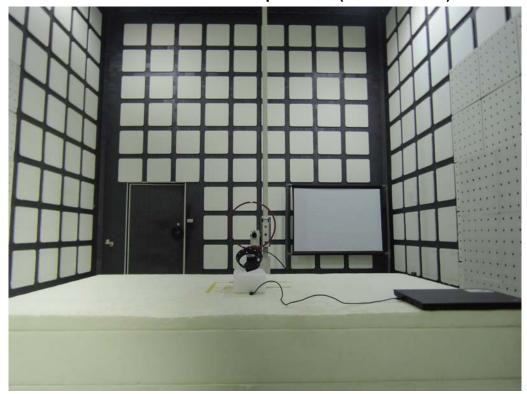
Radiated Emission Set up Photos (Below 1GHz)
