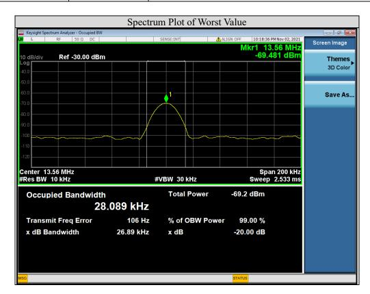
Note: The characteristics of the signal will cause the spectrum analyzer RBW to be unable to set comply with 1~5% emission bandwidth. However, set the RBW:10KHz for spectrum analyzer already can meet the emission is contained within the operated frequency band designated in the rule section, so no longer continue to reduce RBW setting.
