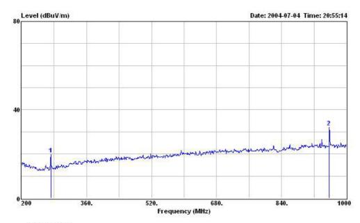
Condition: 3m LOG-9111-221 HORIZONTAL EUT: GSM/GPRS handset 900/1800/1900 MHz
