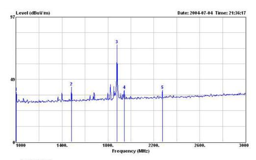
Condition: 3m HORN-ANT-6821 HORIZONTAL EUT: GSM/GPRS handset 900/1800/1900 MHz
