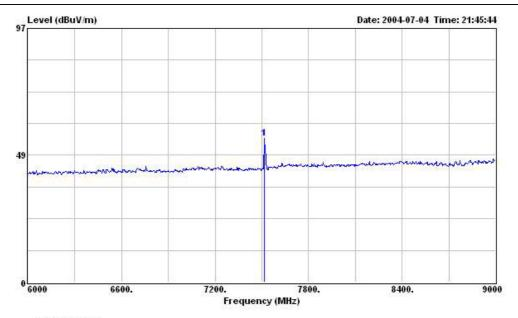
Condition: 3m HORN-ANT-6821 HORIZONTAL EUT: GSM/GPRS handset 900/1800/1900 MHz
