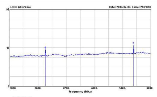
Condition: 3m HORN-ANT-6821 VERTICAL EUT: GSM/GPRS handset 900/1800/1900 MHz
