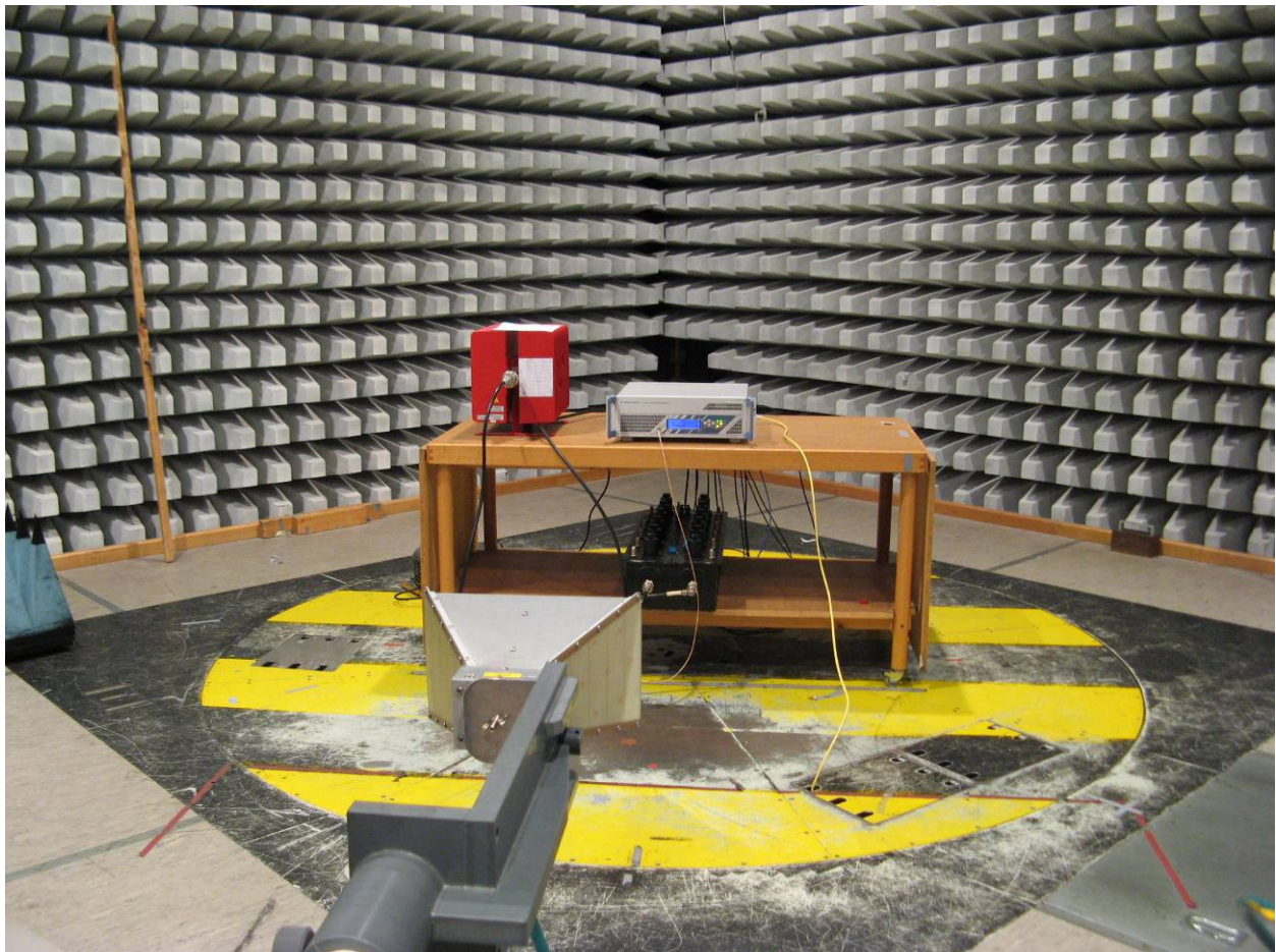
Figure 6-4: Test setup for radiated emission measurement, 1 - 10GHz
