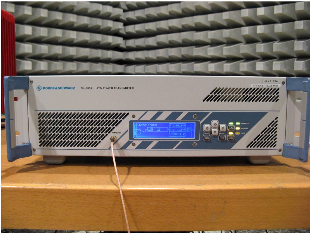
Figure 4-1: SLV8100A in the EMC chamber for Emission Tests front view
