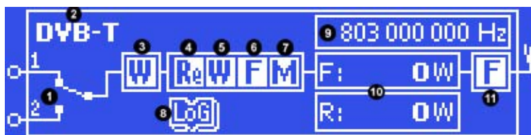
Fig. 2 Possible error indications on the display of the R&S SX801 (front panel)
