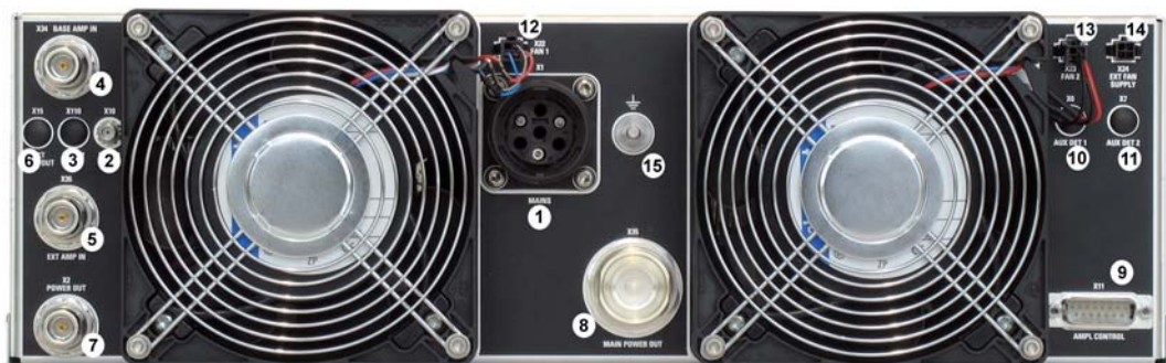
Fig. 3 Rear-panel amplifier connections (here: extended amplifier)
