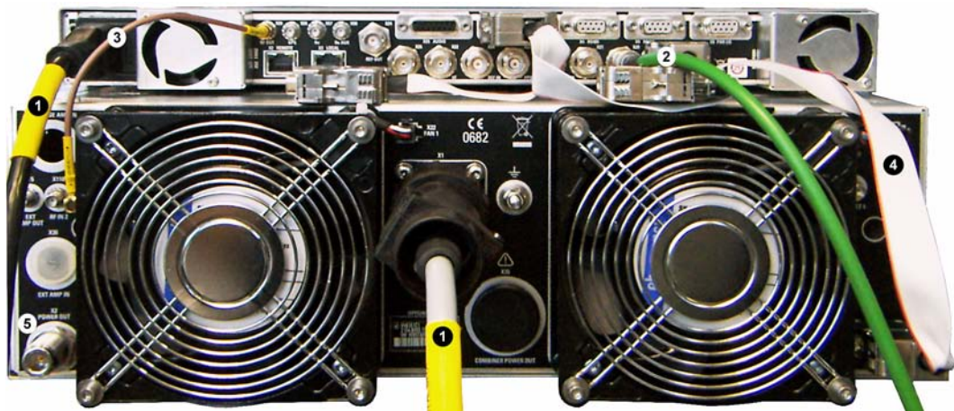
Fig. 1 Example: Cabling the R&S SCV8301E
