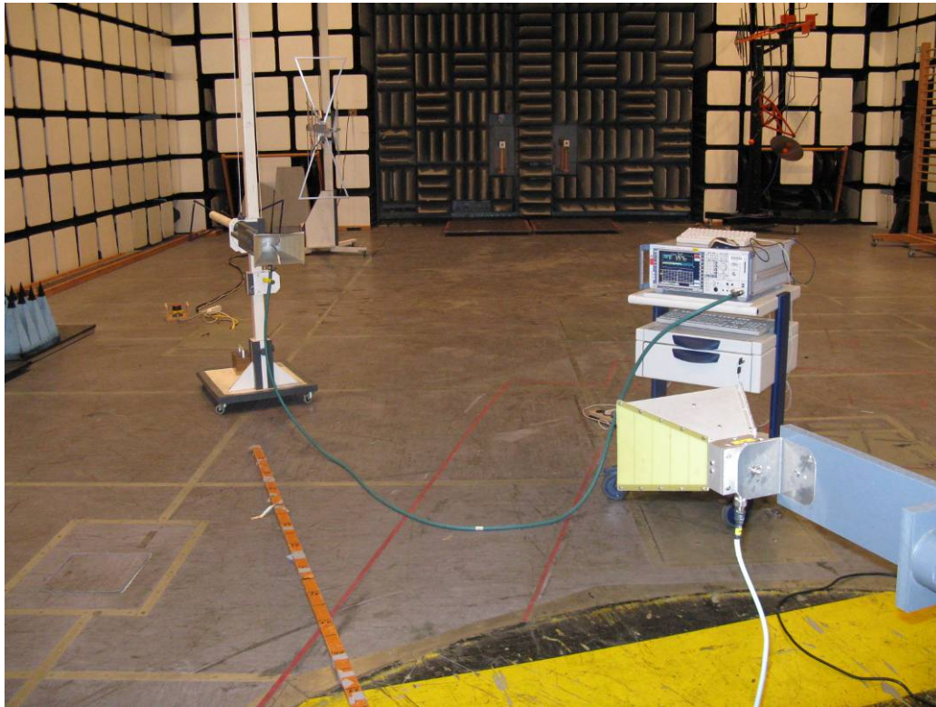
Figure 6-9: Test set-up for the Dipole substitution
