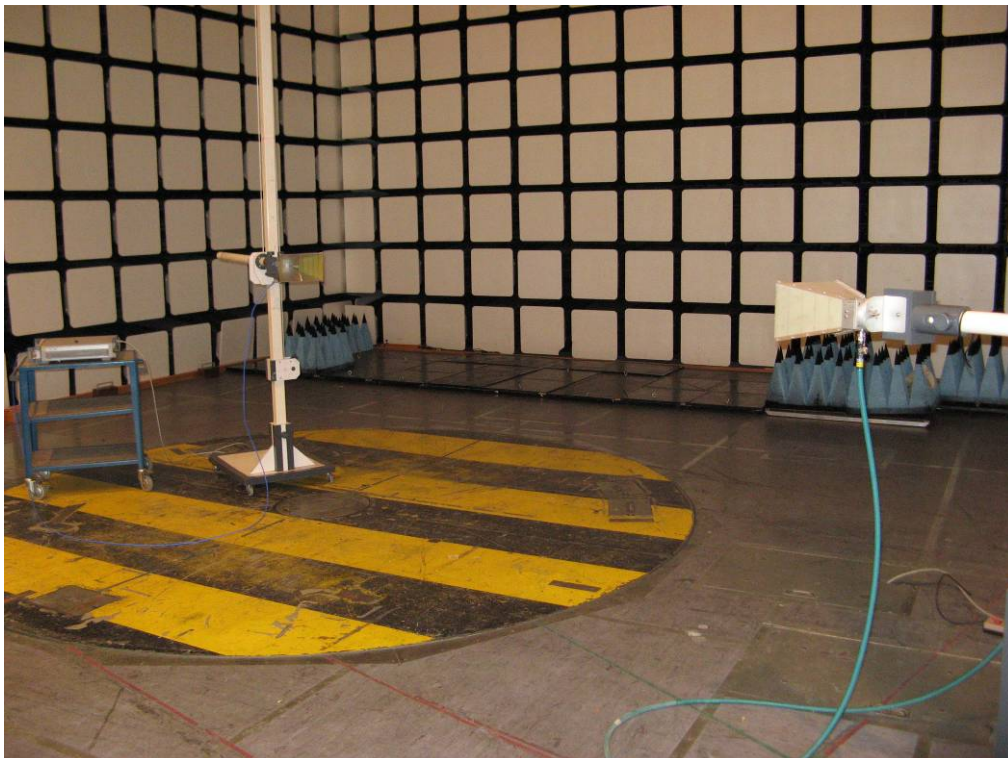
Figure 6-7: Test set-up for the Dipole substitution
