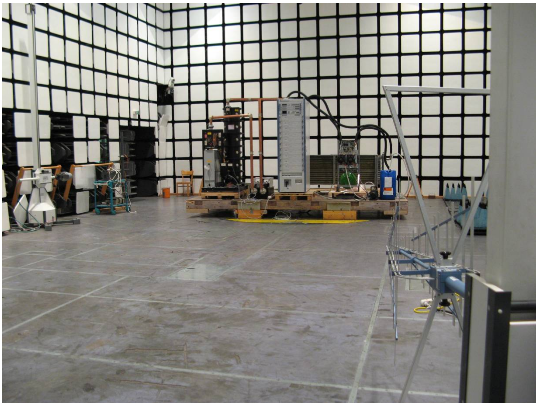
Figure 6-1: Test setup for radiated emissions measurement
