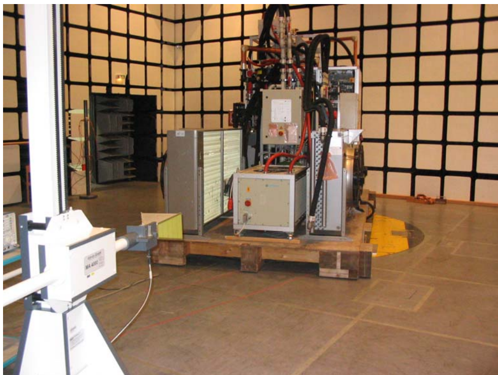
Figure 5-6: Test setup for radiated emission measurement, 1 - 10GHz
