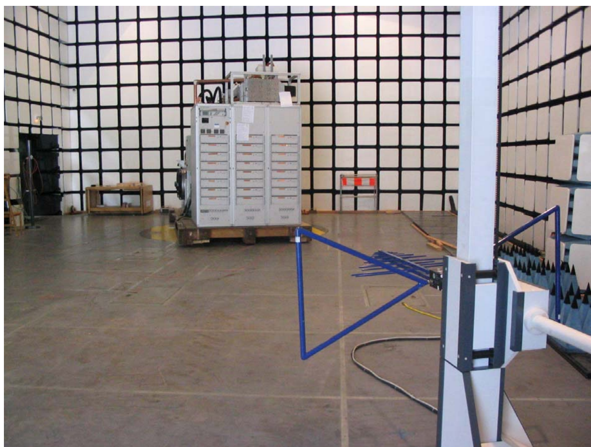
Figure 5-3: Test setup for radiated emission measurement, 30 MHz to 1000 MHz
