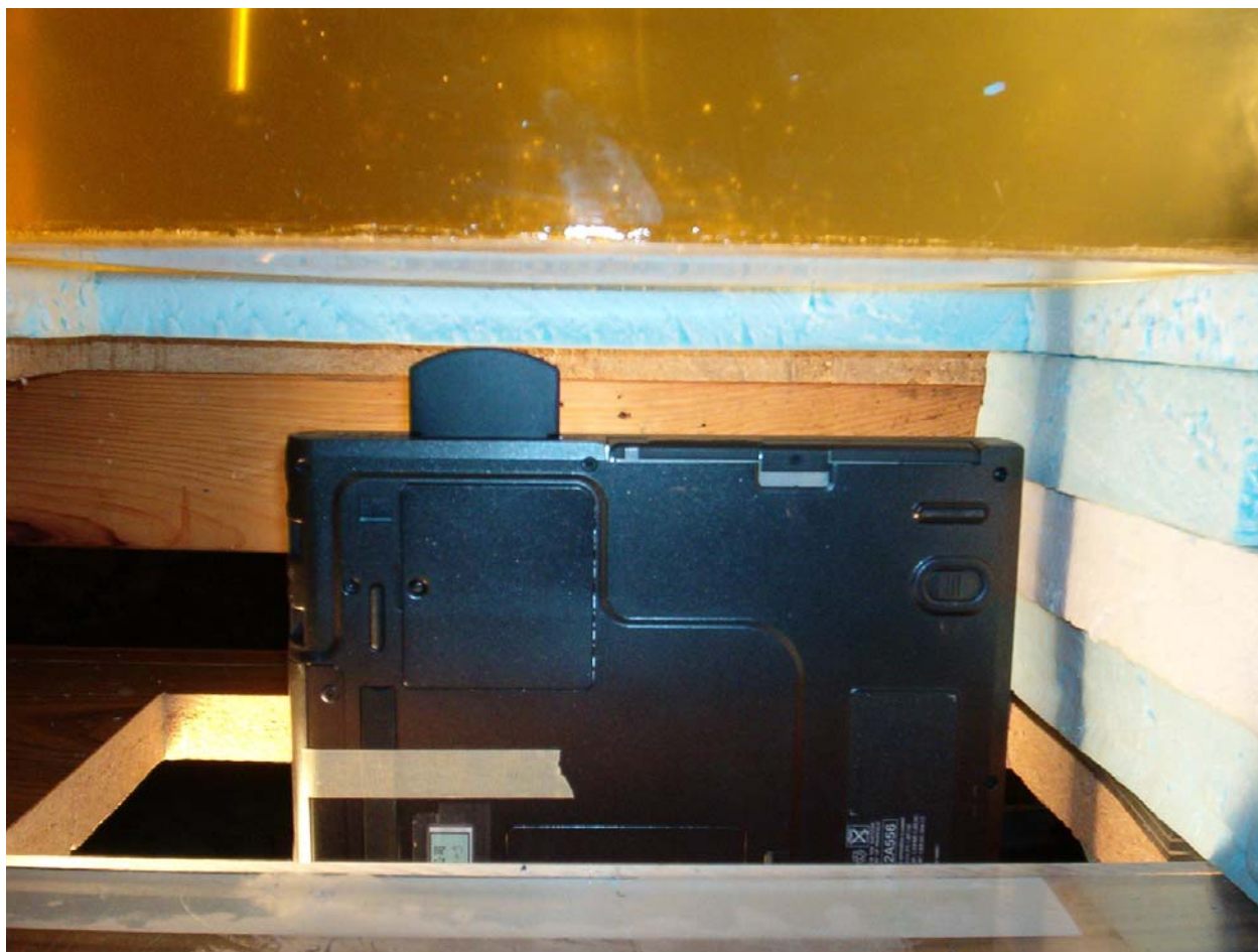
Fig. 6. Photograph of the Accton Technology Corporation WLAN Mobile Adapter inserted into a Compaq portable computer (as in Fig. 1) placed with the adapter edge at 90^\circ and separated from the bottom of the phantom by 2.5 cm for "end-on" testing of SAR. As in Fig. 5, here too, a Styrofoam block is used under the base to prevent bending of the 2 mm thin base of the phantom.
