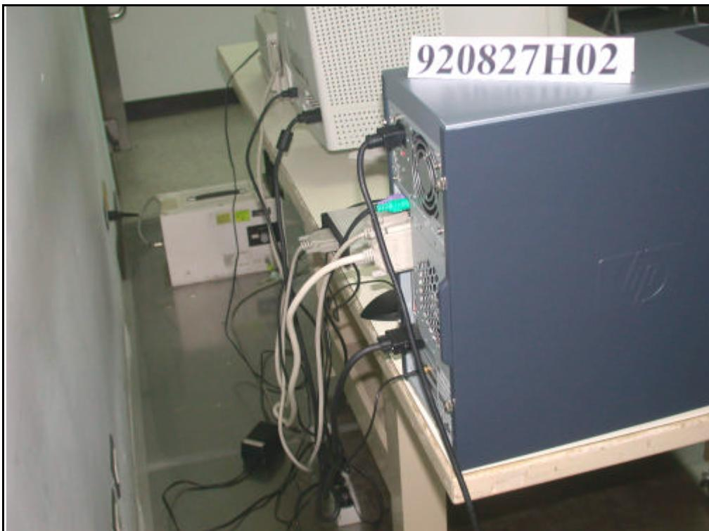
RADIATED EMISSION TEST (For Compaq PC)
